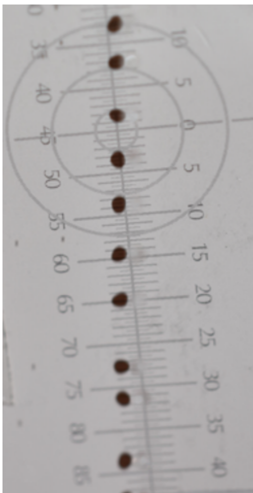
Fig. 2 Shadows of 1.8 mm drops against index card with millimeter length scale, generated using first droplet generator design
