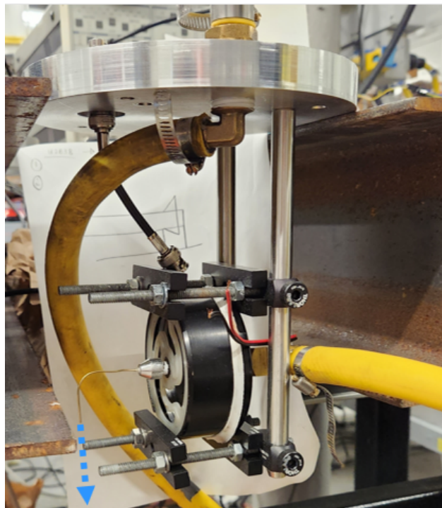
Fig. 31 Drop Generator modified to eliminate collection tank
